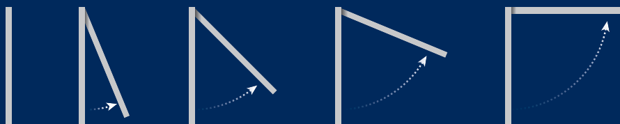
The SupaScape™ fire egress system has an outward opening functionality. Top Hung option shown.
