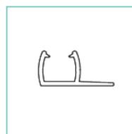
6mm Vertical Flap with 15mm Leg PGFVL15-6
